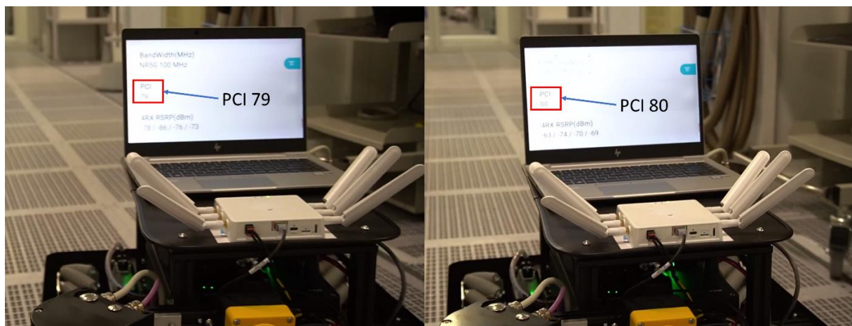
Figure 16: Snapshots of the evaluation of AGV operation when handovers happen during the motion of the robots (the Physical Cell ID (PCI) changed from 79 to 80).
