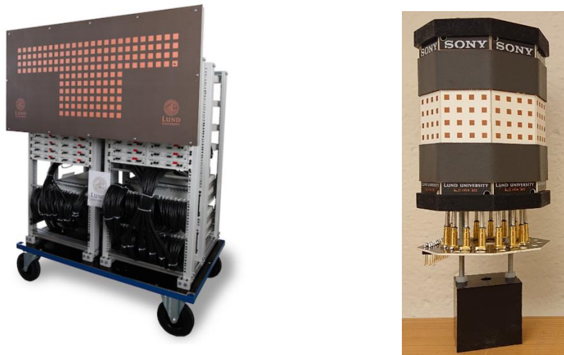
Figure 10: Front view of the 3.7 GHz LuMaMi system (left) and mmWave propagation sounder (right).
